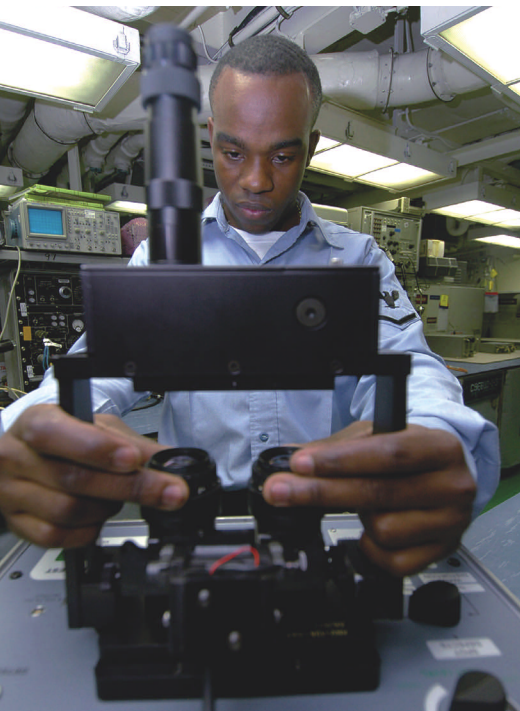
Aviation electronics technician Sheridan Lee calibrates a pair of night-vision goggles aboard a ship. NSWC engineers wrote the calibration procedure that Lee follows. Courtesy of US Navy.
